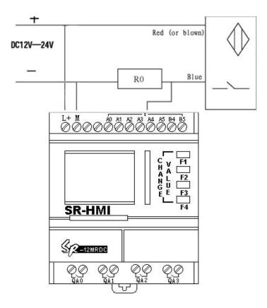
To the same type approach switch, its connection principle is alike. For NO and NC type approach switch, their difference is output relation when it near to
