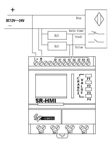
Example 2: Inductance double line AC approach switch with SR Structure chart:
